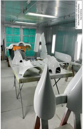
I've started putting some of the airplane back together again. Cowling, spinner, ailerons, wingtips, inspection covers. I'm holding off on the flaps and tail feathers until they get around to painting the colors because I don't want them to be in the way, or subject to overspray because of close proximity to the colors being applied. The paint scheme is actually a paint mask, and I'll be helping to lay that out.
