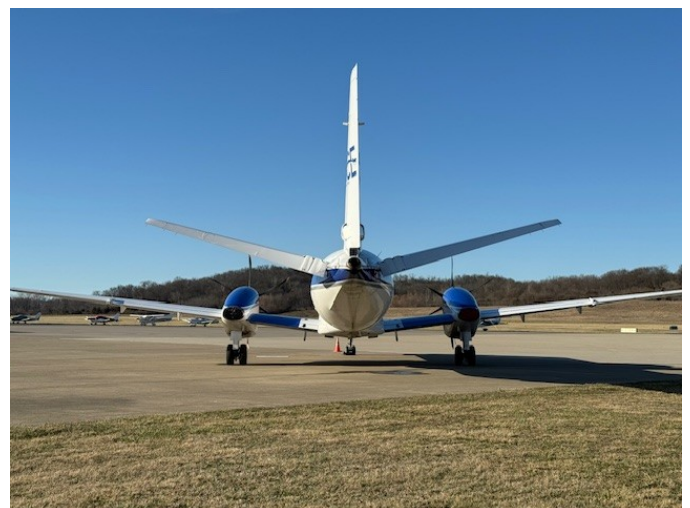
Left and lower right, a Saab 2000 parked on our apron afternoon of Feb 29, something we don't see very of-ten! I was so taken and distracted, I almost forgot to go flying. What a striking and beautiful aircraft! Check out that dramatic dihedral horizontal stab and those 6 blade props! Photos: ed.
