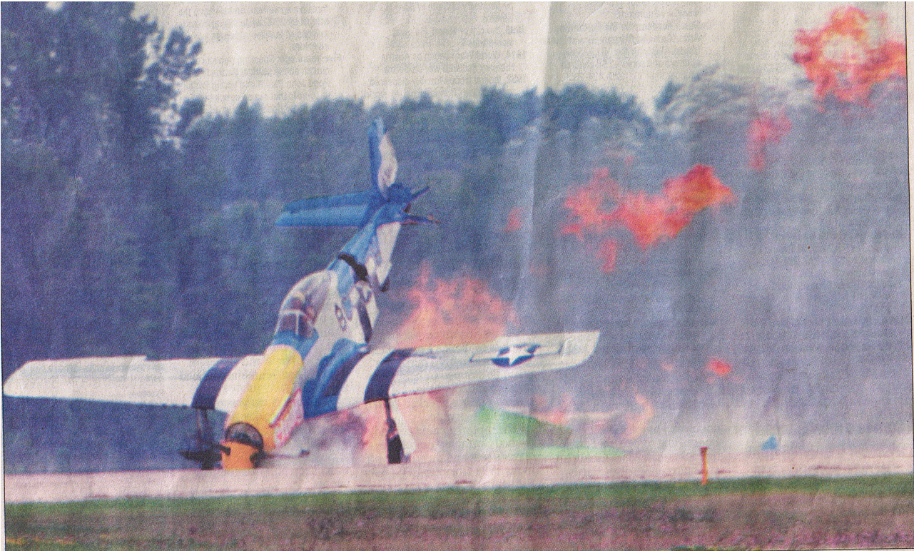
The following plane appeared to attempt a go-around and roll over due to torque
