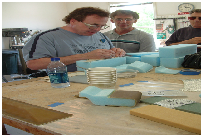
John secures canard template to foam, 2
