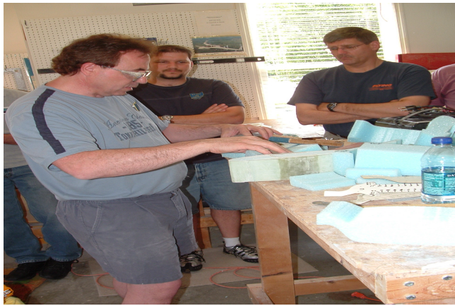
Cut core in foreground, layed up core next to John's hand
