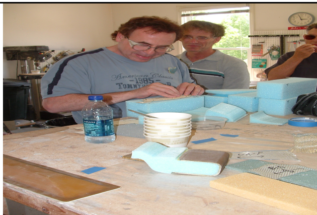
finishing canard template, preworked core with spar in foreground with Uni and BID samples and last-a-foam
