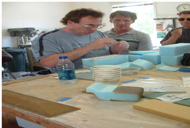
John secures canard template to foam
