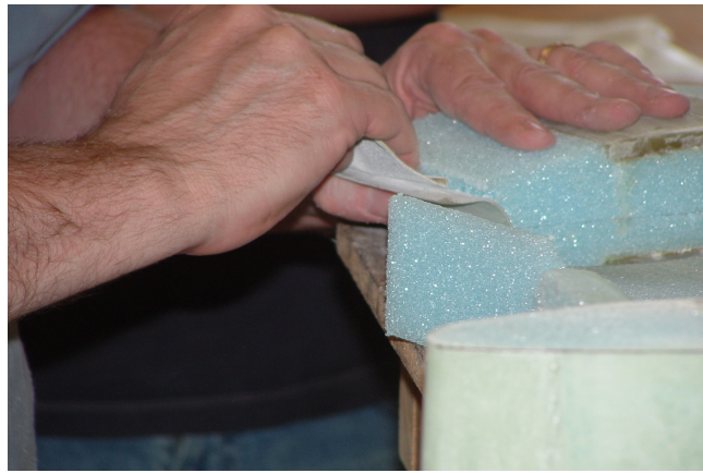
Layed up core, after carving off support tab, sanding for trailing edge lay-up
