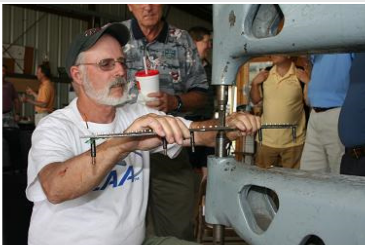
Brian demonstrating the process of Riveting the spars
