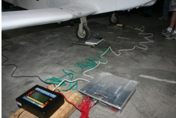
These are heavy duty scales designed for Sports cars or heavy aircraft
