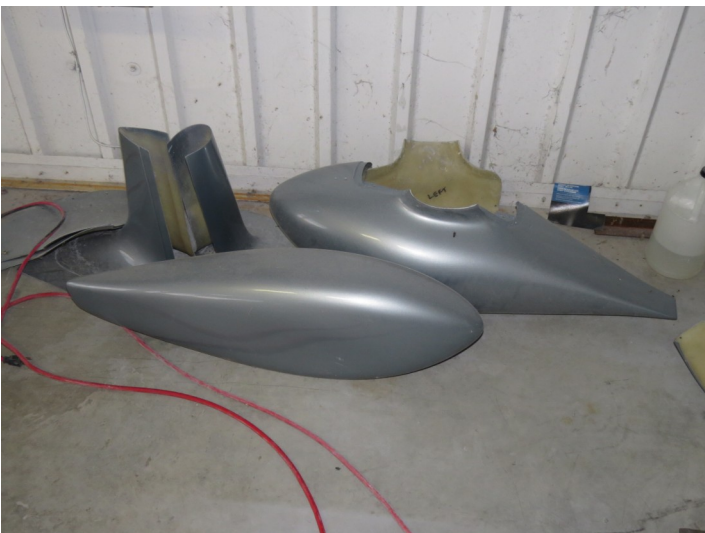
Above left: wheel pants and strut fairings ready to install. Should make it go like greased lightning!
