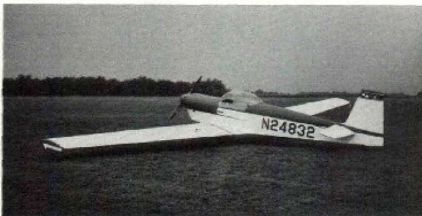
The Miller Sport Plane at the Philadelphia Glider Council Airport just prior to its first flight. Notice the slick fairings for the wingtip wheels.
