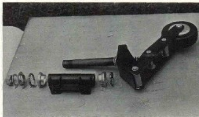
Tailwheel unit — yep, those are bicycle bearings and races. Total weight is 4½ pounds.
