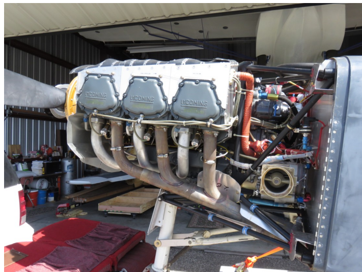
Above: Here's the thing that really makes it fly—an IO-540. How about 300 HP ! All it takes is horsepower and $$!
