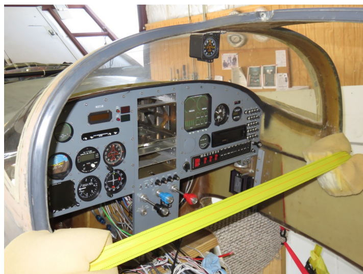
Below: A nice looking panel, a hybrid of steam gauges and glass. This is the part that can really eat up time. Almost done!
