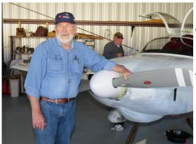
Ken Jones, in Hangar T9-B is another two-project juggler. Ken spent 18 months in a massive restoration of a Glasair involved in an incident by the previous owner. He converted it from a tail dragger to tricycle gear. It is powered by a Lycoming O-360. First flight was in 7/2016. He is currently working on new fairings and the transponder. Check out the beautiful interior (inset photo). Ken's other project is a Sonex which he has been flying for some time. He is com-
