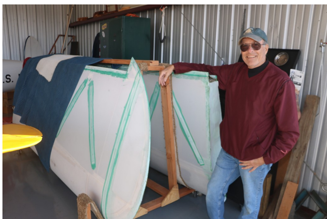
Shown at left is Al Kenkel with a set of Ercoupe wings he recently acquired. These are fabric covered and fabric was attached with Stewart Systems Ekobond fabric cement. Al says he plans to go ahead with the Stewarts Water-bourne coatings to maintain compatibility with the cement. Having done my latest project in Stewarts, I can vouch for its ease of application. Nothing like a spare set of wings! Great, Al!!
