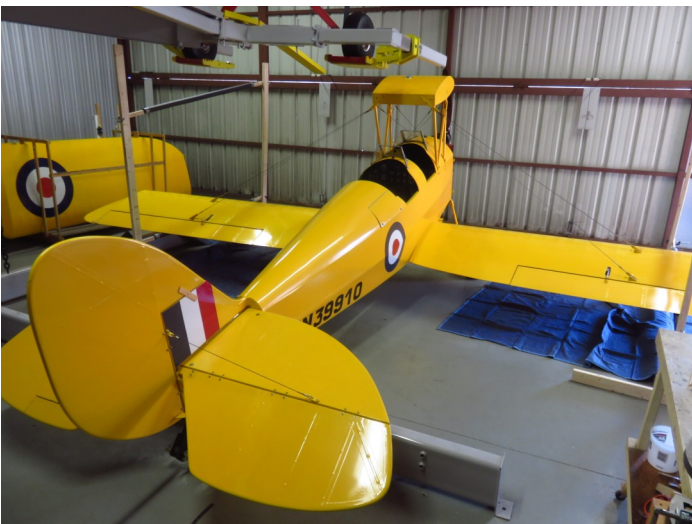
This was a big moment, as the wings start to go on my Tiger Moth project. This is just a temporary mounting of the lower wings just to verify aileron pushrod length. The wings have removed temporarily, and final riveting of the pushrods is done. Next the upper wings go on followed by replacement of the lower wings. Of course I had to enlist the aid of my wife Nancy to make her feel part of the project. (Not that she didn't already, having given up most of her laundry room for over 10 years!) Thanks Nancy! Photos: ed.
