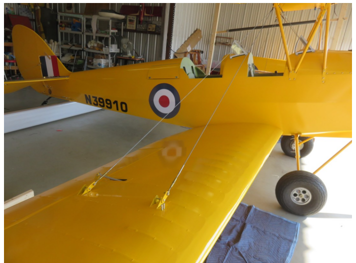
This was a big moment, as the wings start to go on my Tiger Moth project. This is just a temporary mounting of the lower wings just to verify aileron pushrod length. The wings have removed temporarily, and final riveting of the pushrods is done. Next the upper wings go on followed by replacement of the lower wings. Of course I had to enlist the aid of my wife Nancy to make her feel part of the project. (Not that she didn't already, having given up most of her laundry room for over 10 years!) Thanks Nancy! Photos: ed.
