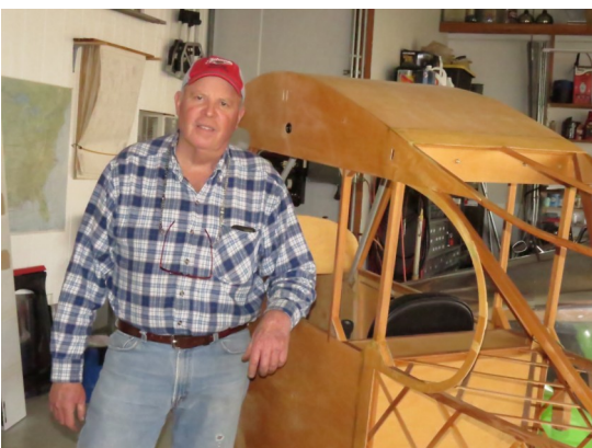
Upper left, Note the geodetic construction, universal for Fisher aircraft, like a Wellington Bomber
