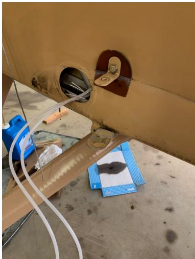
Seen left, besides struts and wires, the pitot/static lines had to be disconnected on both ends from fuselage and from pitot/static tube and aileron pushrods had to be disconnected at fuselage and at lower ailerons.
