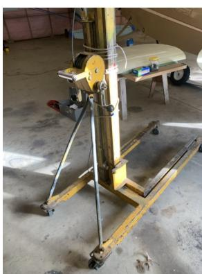
*Seen left a mechanical fork lift. A drywall lift could be modified for supporting the wing. The tail is raised to level the wing to the forklift.*
