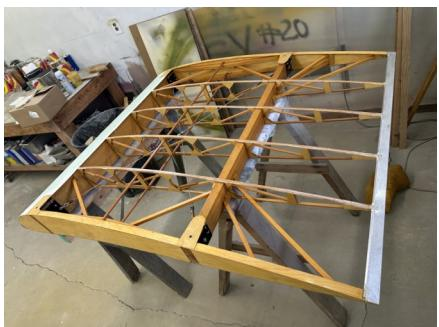
*Left is the uncovered center section, careful inspection revealed no condition issues.*
