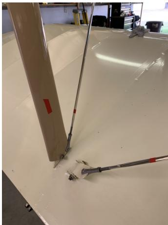
Ailerons were removed first, then removal of all cotter pins (lots of them!) followed by marking wires and struts with colored tape. Red tapes=port side, green tapes= Starboard side. Tape is placed on lower portion of wire or strut to aid in orientation.
